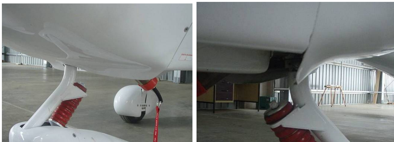
Figure 56: Lip to aid cooling as installed on a Jabiru.
