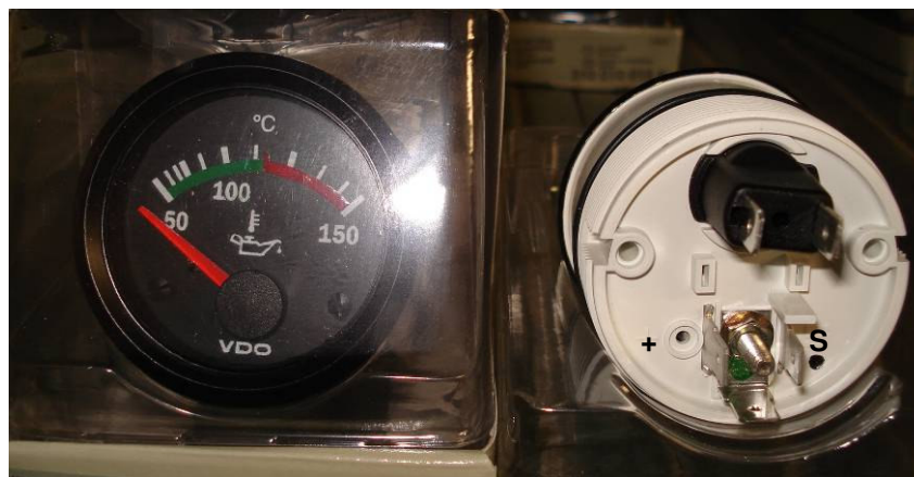
Figure 18. Oil Temperature Connections
