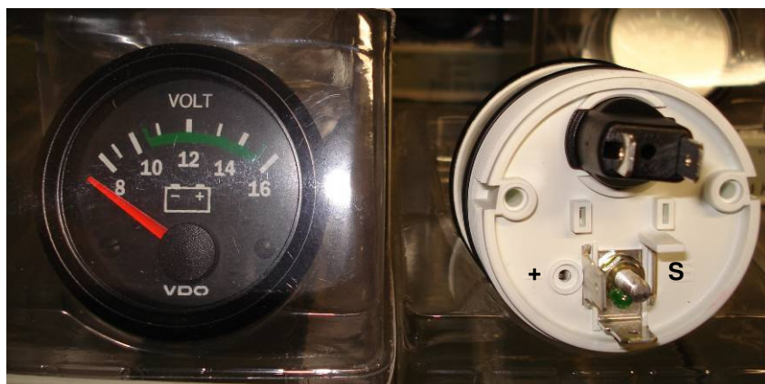
Figure 21. Voltage Gauge Connections
