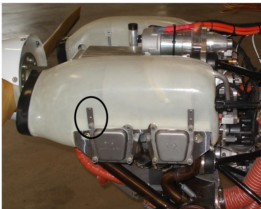
Figure 31 – Air Duct Hard Point Reinforcement
