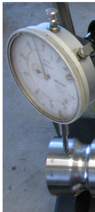
Figure 45 – Dial Indicator Position for Crankshaft & Prop Flange Run Out
