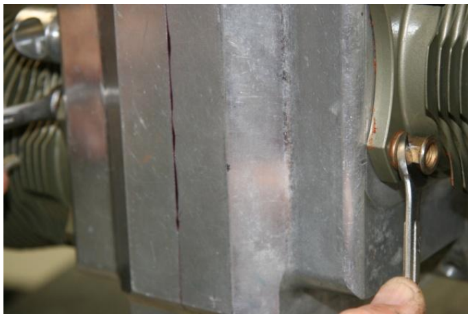
Figure 156 – Tightening, Locking &amp; Marking Through Bolts
