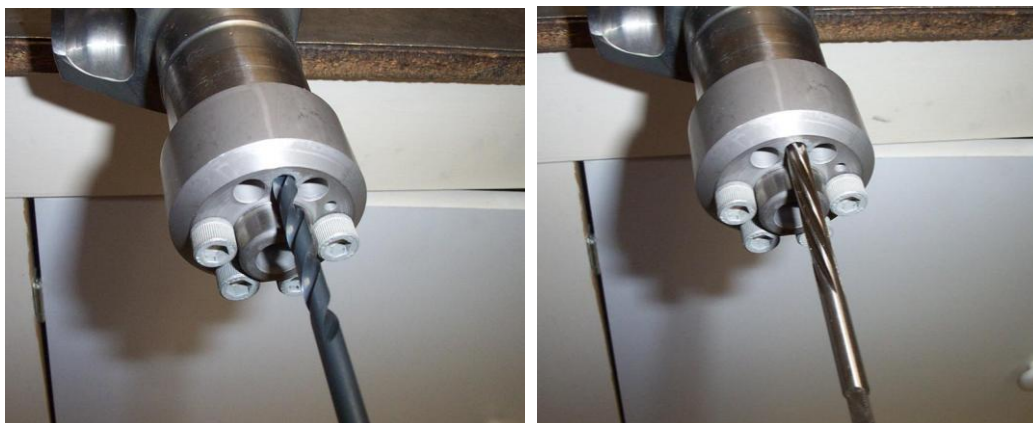
Figure 208 – Drilling & Reaming Crankshaft – ILLUSTRATION ONLY.
