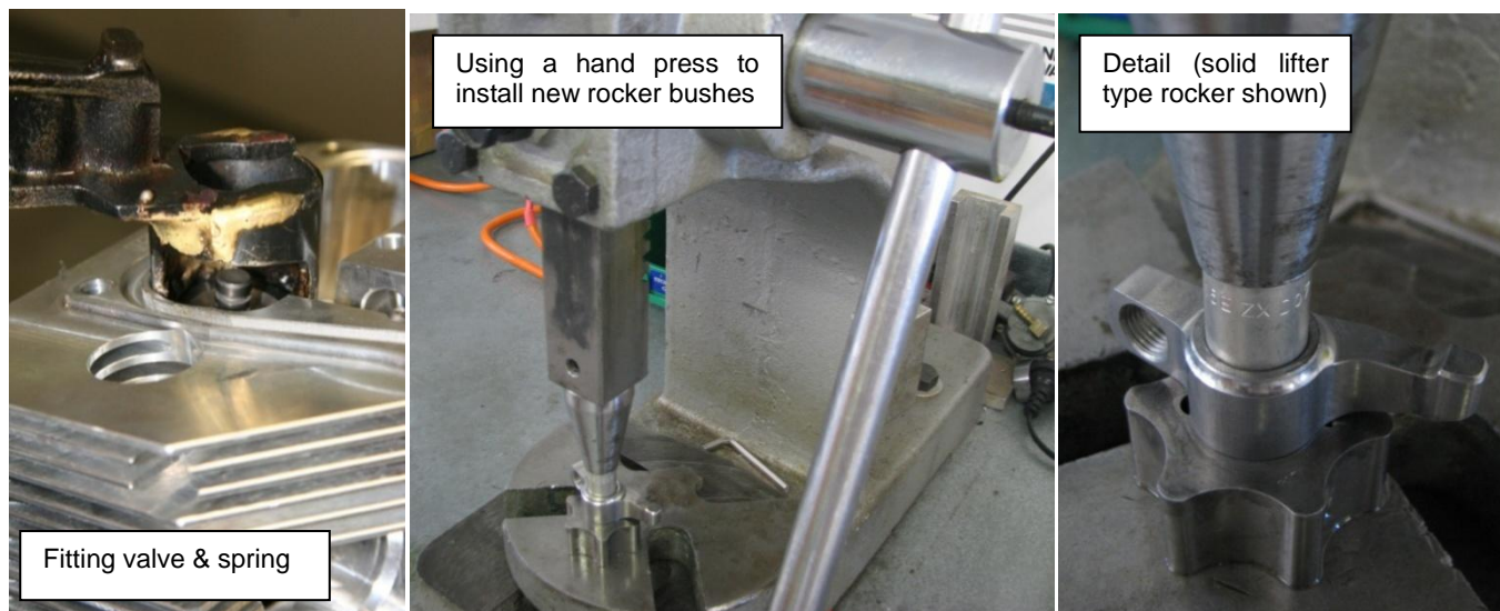
Figure 141 – Fitting Valves to Head, Fitting Bushes to Rockers
