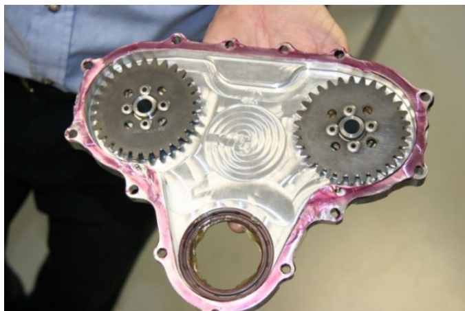
Figure 167 – Fitting Distributor Case &amp; Setting Timing
