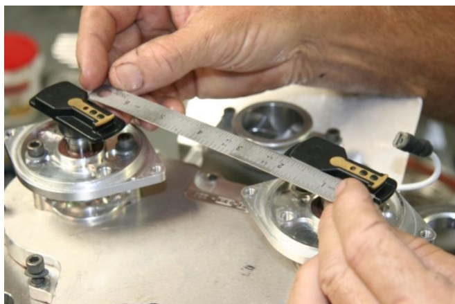
Figure 169 – Checking Rotors, Tightening Distributor Case
