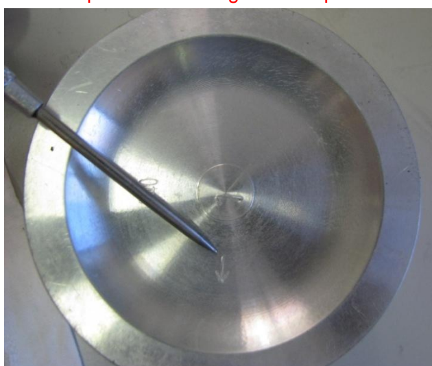
Figure 128 – Thrust Direction Markings For Pistons
