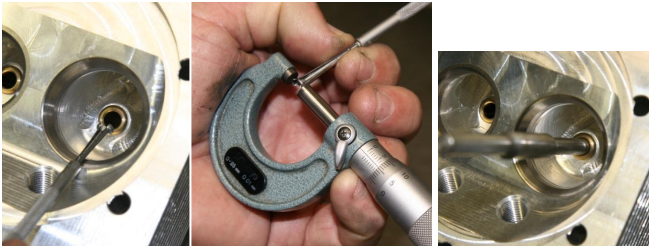
Figure 89 – Measure Guide Wear (Telescopic Gauge Left & Middle, Go-No-Go Gauge Right)
