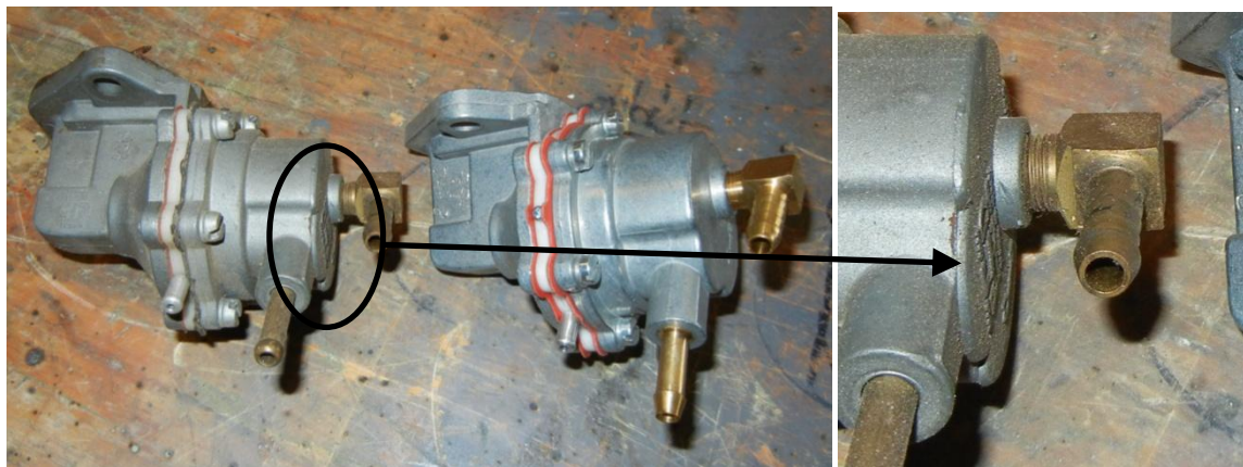
Figure 114 – Fuel Pumps (Type 1 on Left, Type 2 on Right)
