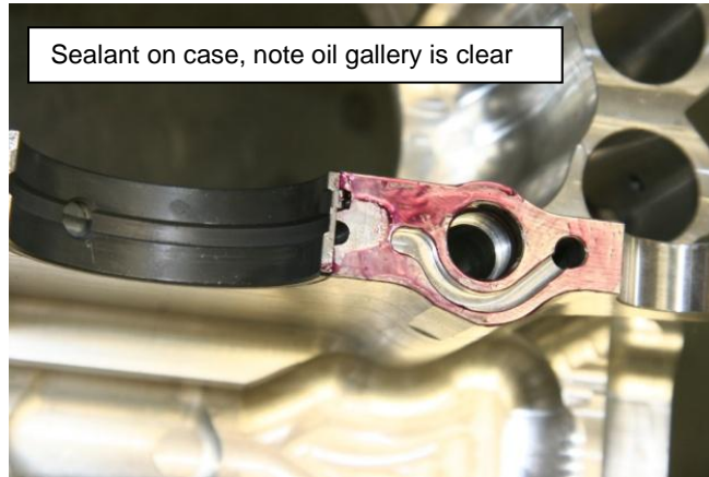
Figure 150 – Applying Sealant to Case, Fitting to Crank
