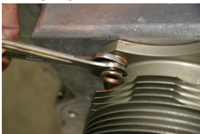
Figure 155 – Tightening Through Bolts With Lock Nuts
