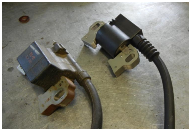
Figure 101 – Different Ignition Coil Models (Honda on Left, Jabiru on Right).
