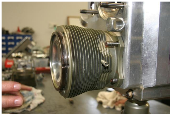
Figure 154 – Fitting Up Cylinder, Inserting Through-Bolts
