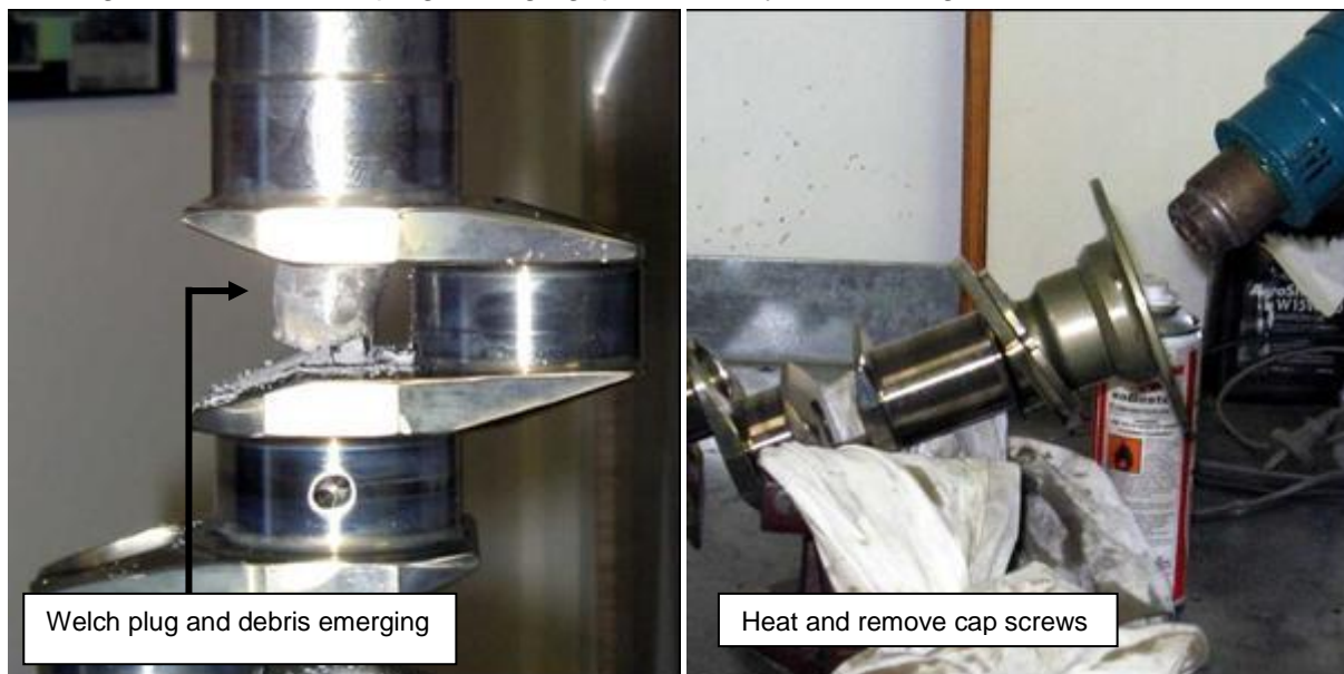
Figure 61 – Welch Plug & Propeller Flange Removal From Crankshaft
