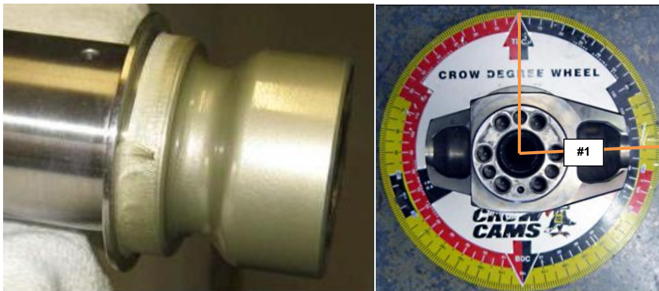
Figure 115 – Crankshaft Painting, Degree Wheel
