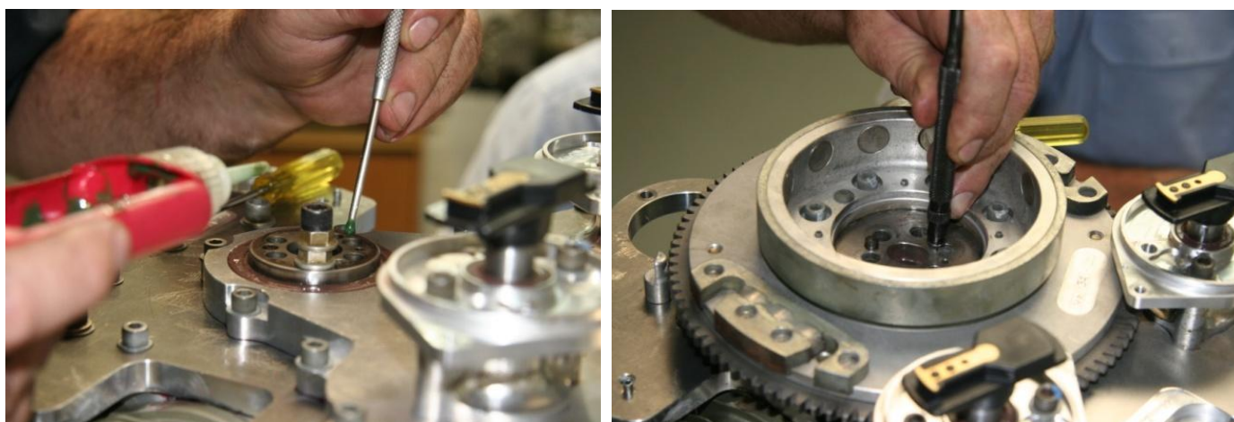
Figure 171 – Applying Loctite, Fitting Dowels.
