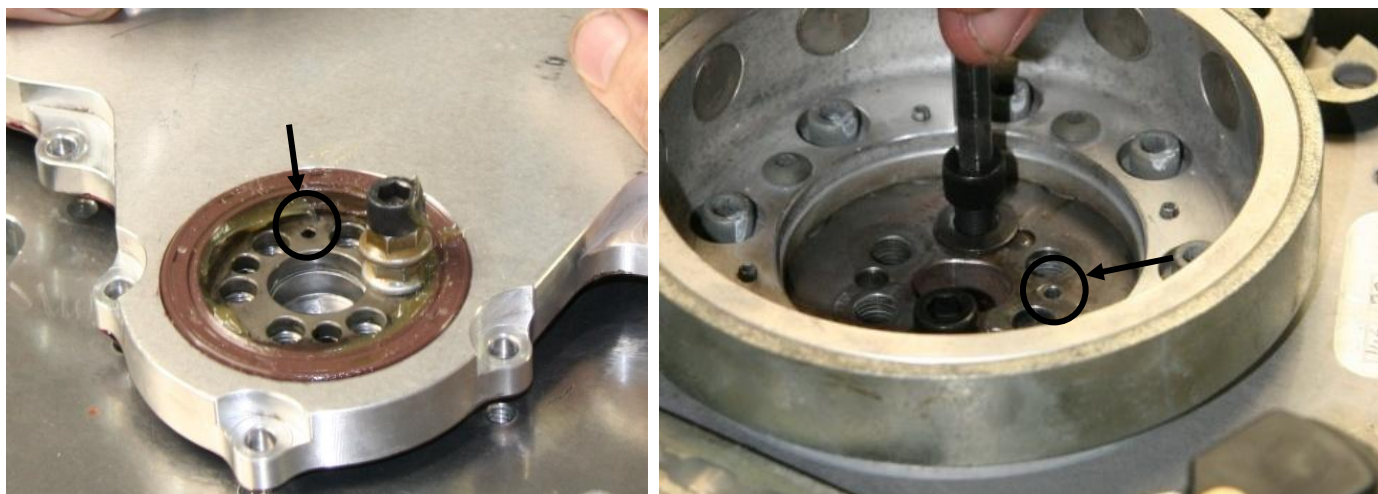
Figure 172 – Flywheel &amp; Crank Timing Marks
