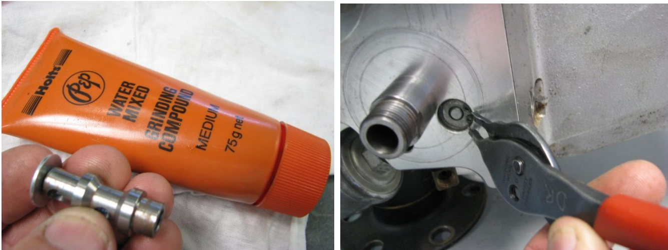
Figure 197 – Lapping Oil Pressure Relief Valve
