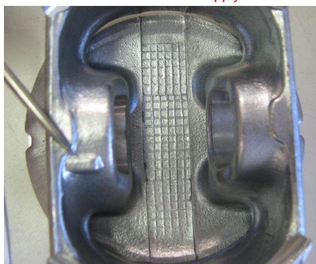
Figure 128 – Thrust Direction Markings For Pistons
