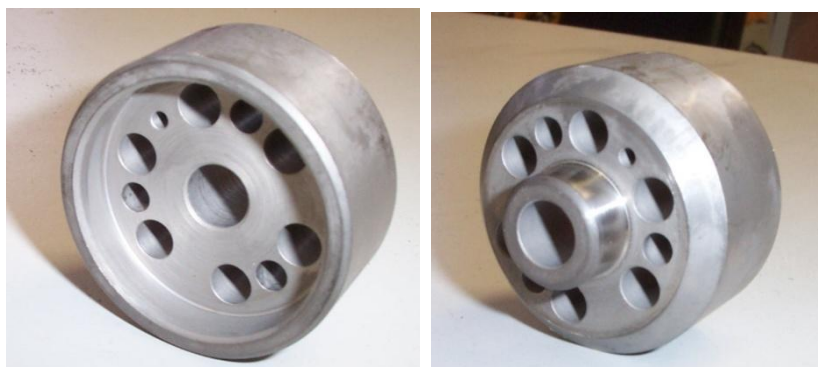
Figure 205 – Drilling Fixture – Crankshaft Side on Left, Flywheel Side On Right
