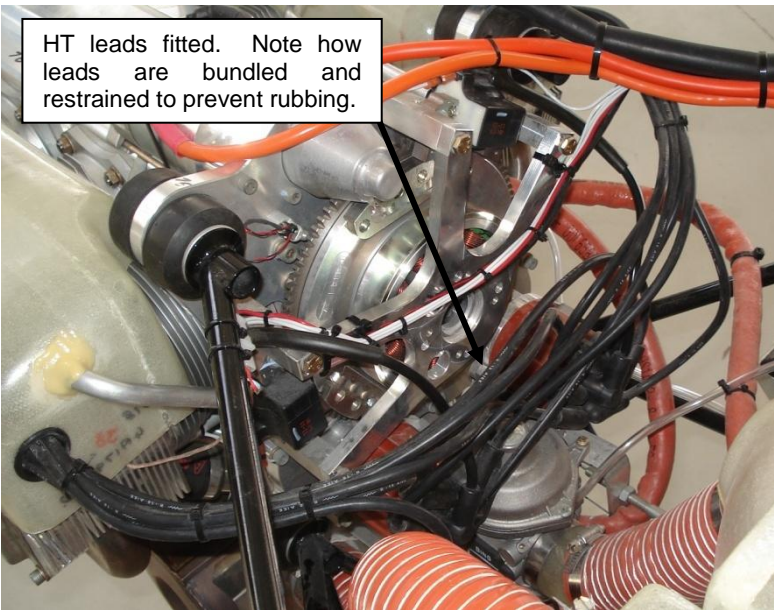
Figure 190 – HT Leads Fitted To Engine REMOVE ENGINE FROM STAND.
