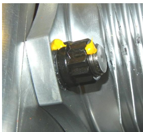
Figure 156 – Tightening, Locking &amp; Marking Through Bolts
