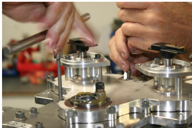
Figure 169 – Checking Rotors, Tightening Distributor Case
